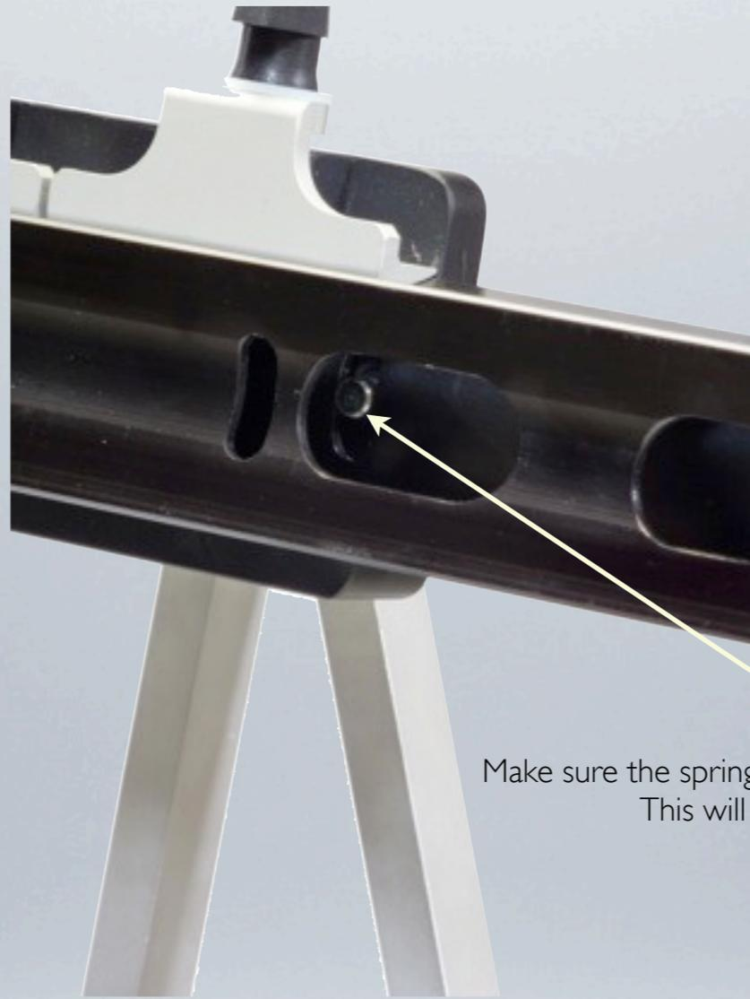
Make sure the spring loaded pin engages the slot on the rail.
