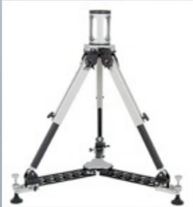
Note: The Explorer Version 1 Tripod looked like this. It had short legs, clamps for feet, and a large spreader base with leveling feet. It was designed like this to make it a quick change-over to a 3-Leg track dolly by exchanging the leveling feet for dolly wheels. It worked well as the jib/trolley support, but it was slow to set up because the spreader base needed to be assembled, and its short legs made it impractical as an everyday tripod.
