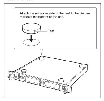
To install the DWR-R02DN in the rack, be sure to remove the attached feet.
